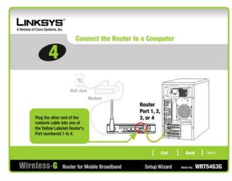
Figure 6-6: Connect the Router to a Computer Screen, continued
